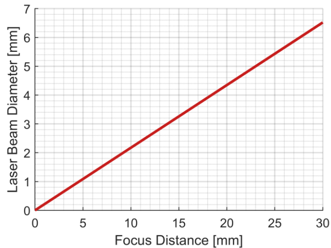
Figure 3: Spot diameter in respect to the distance from the focal length of 63.5 mm and 13.8 mm as initial spot size.
